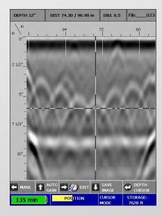
Locate targets in real-time using 2-dimensional data collection mode.
