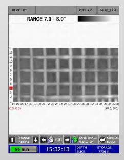
Identify complex characteristics in concrete with the 3D data collection mode.
